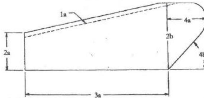
No more than (3) Spoiler supports permitted. Front edge of supports must be in line.
